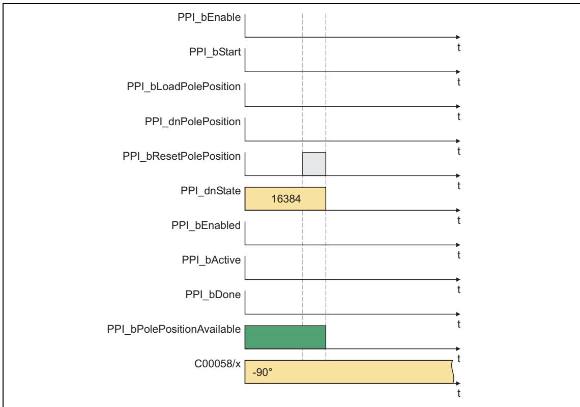
[11-56] Signal characteristic 3: Reset pole position
