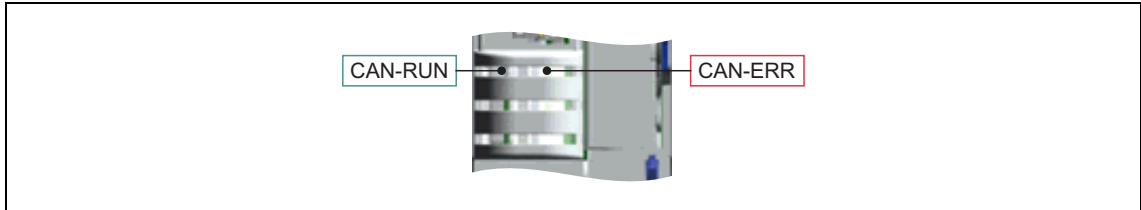
[9-2] LED status displays CAN-RUN and CAN-ERR
